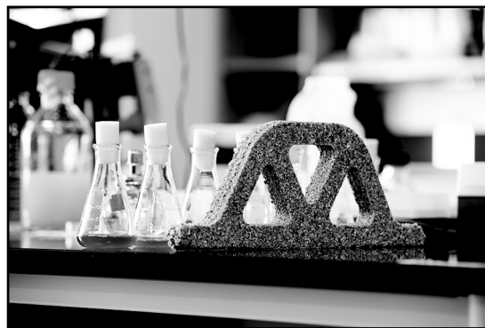
An arch made from living building materials in Dr. Srubar's lab.
